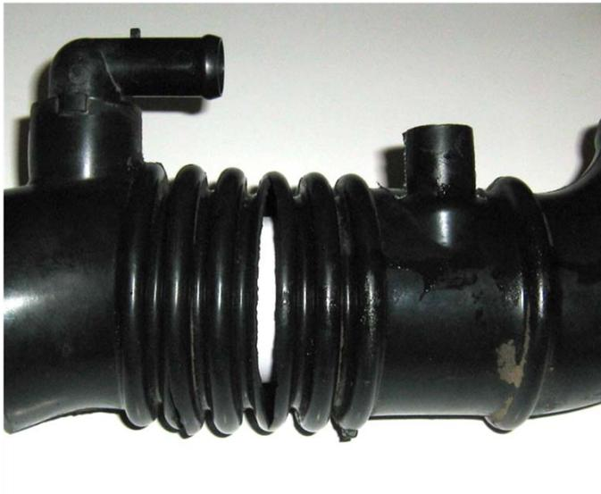
**Picture 4 :** Flex hose with crack. We have put some white paper in the tube to make the crack more visible.
