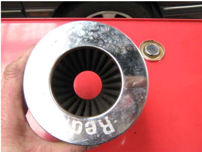
Figure 10: The shiny disc has damaged the grate, destroying the airmass sensor.
