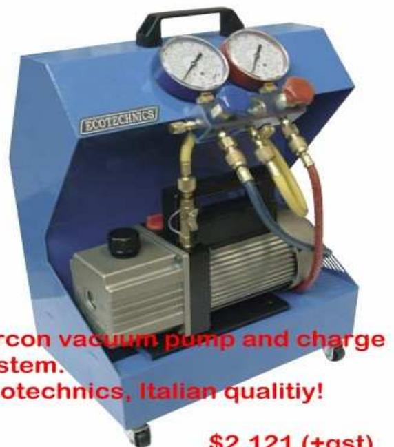
**Aircon vacuum pump and charge system.
