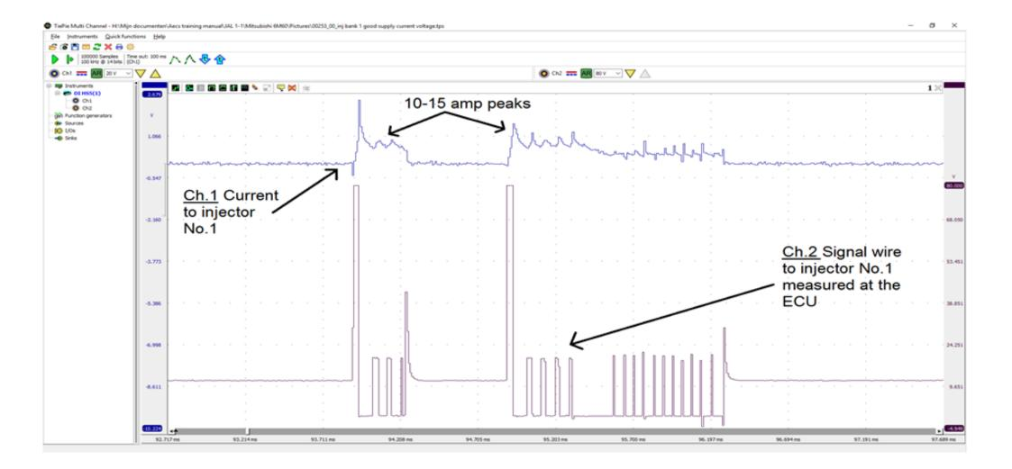
Picture 3: Scope recording showing correct injector current control.
