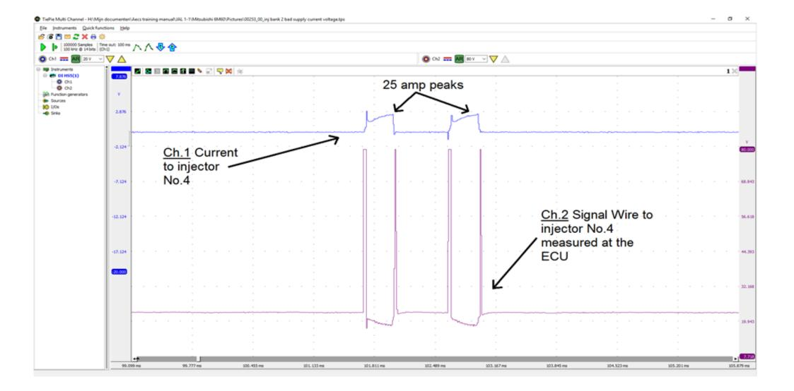
Picture 2: Current and power supply to the injector bank.
