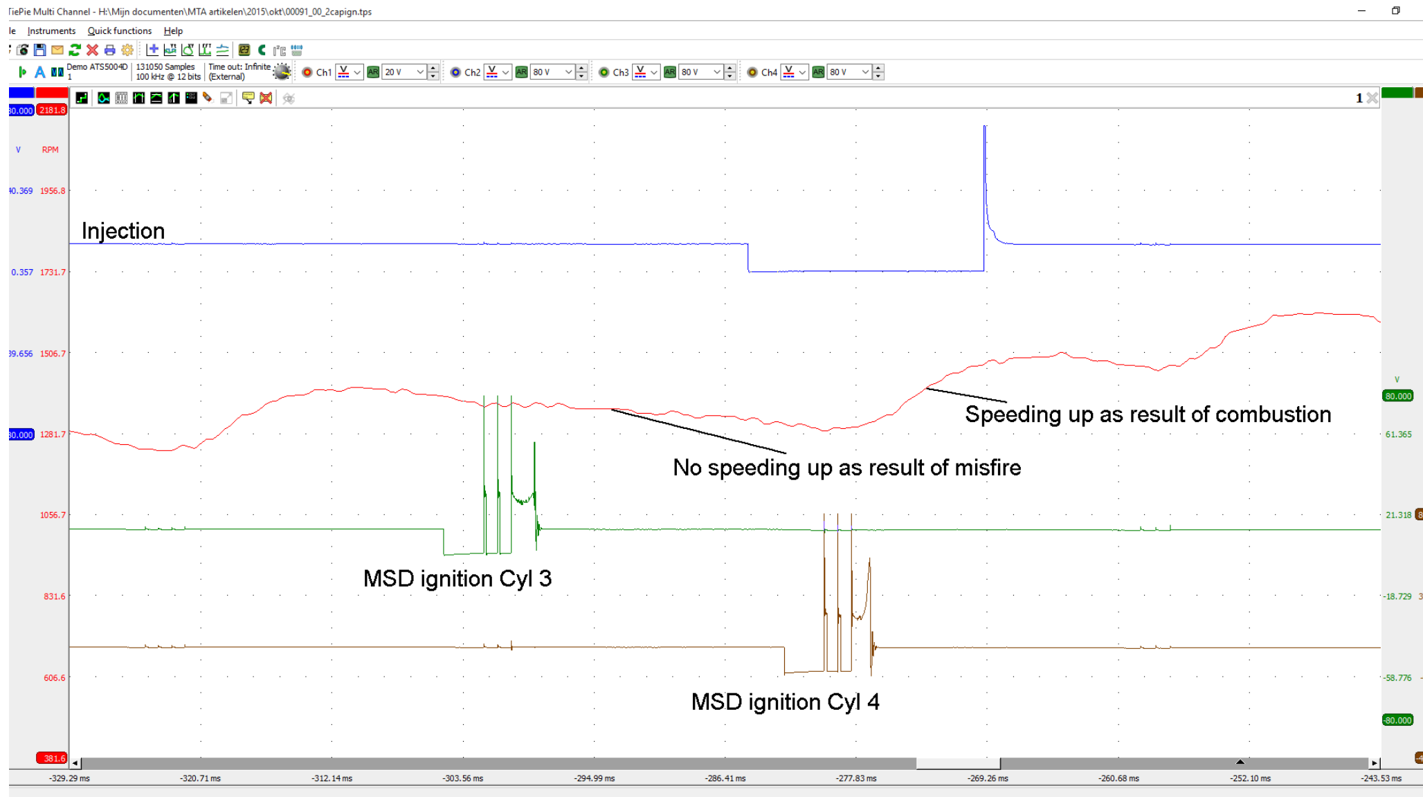
Picture 2: Recording of the crankshaft sensor, Injection and the coils on cylinder 3 and 4 zoomed in.
