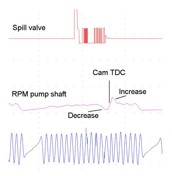
Picture 6: Detail of spill vs pump shaft recording
