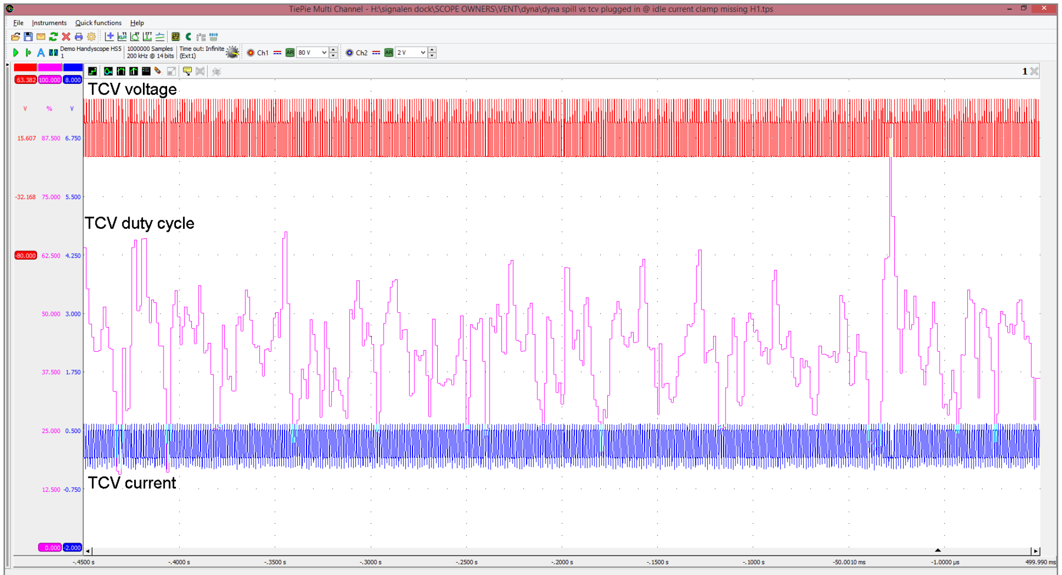
Picture 4: TCV voltage over current, running really bad (warm engine).
