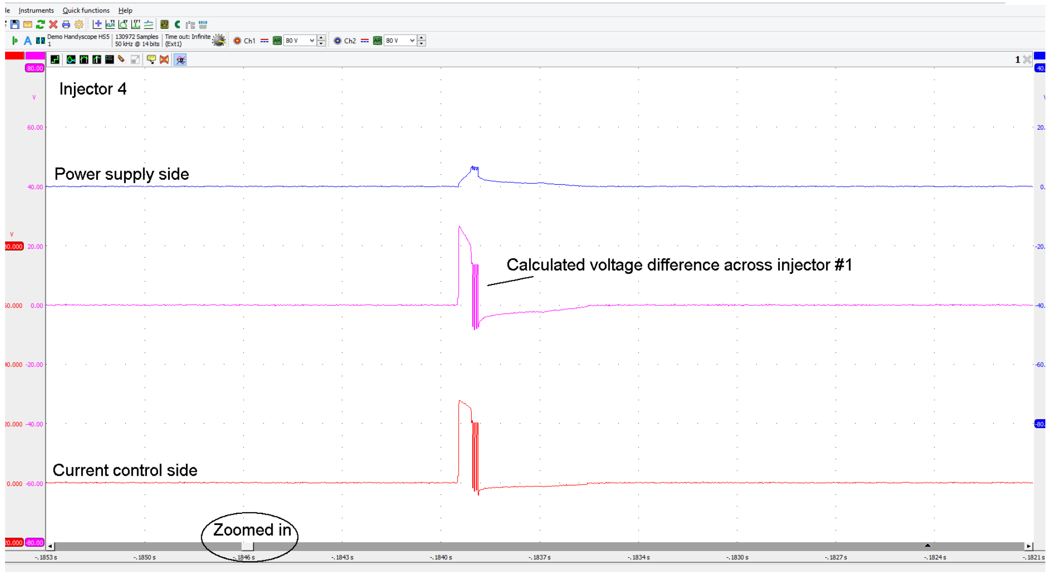
Picture 3: ATS 500XM scope recording, Ch2 connected to injector #4 (faulty) power supply, and Ch1 connected to the injector current control wire.
