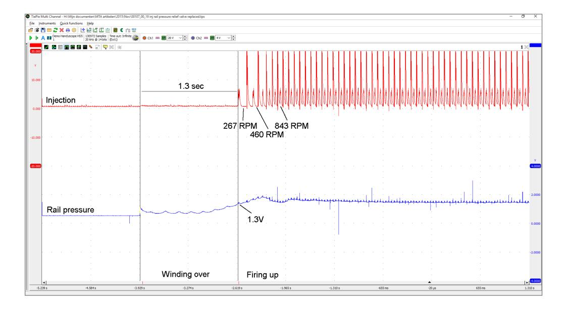
Picture 5:ATS 500XM scope recording of injection vs rail pressure.
