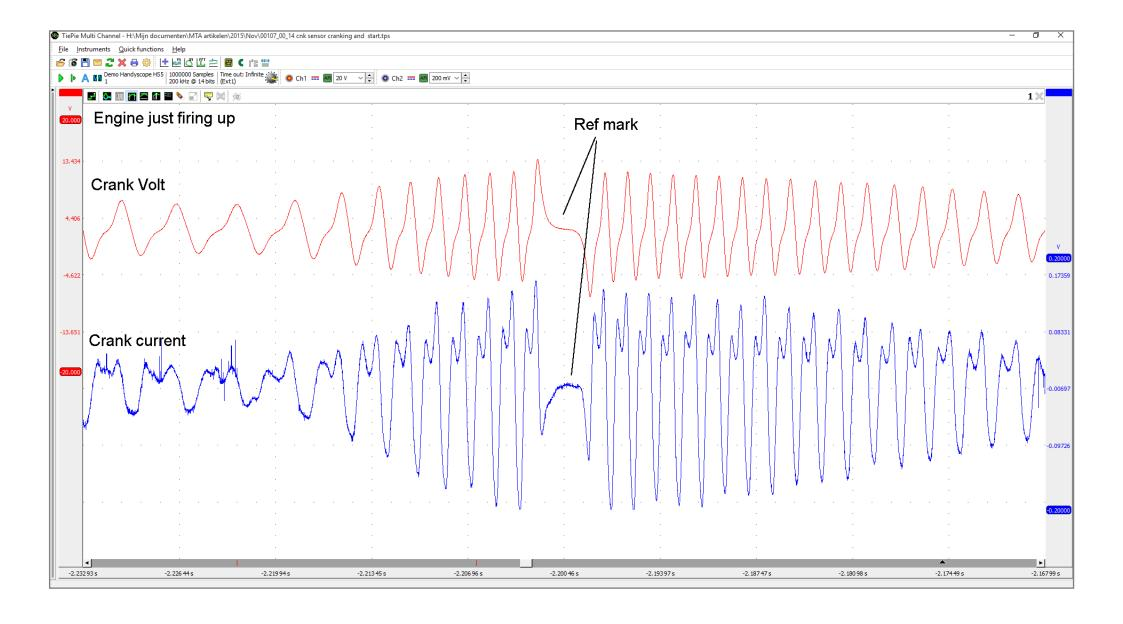
Picture 4: Scope recording zoomed in on 'the engine just firing up'.
