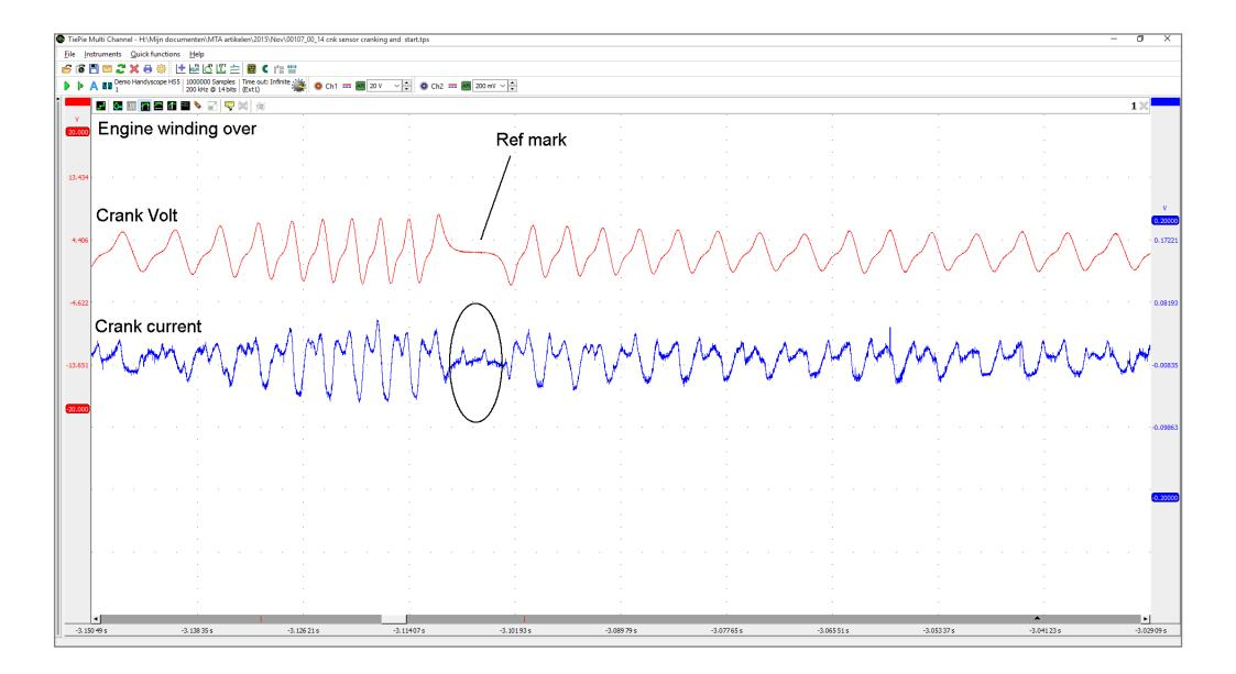
Picture 3: ATS scope recording zoomed in on 'the engine winding over'
