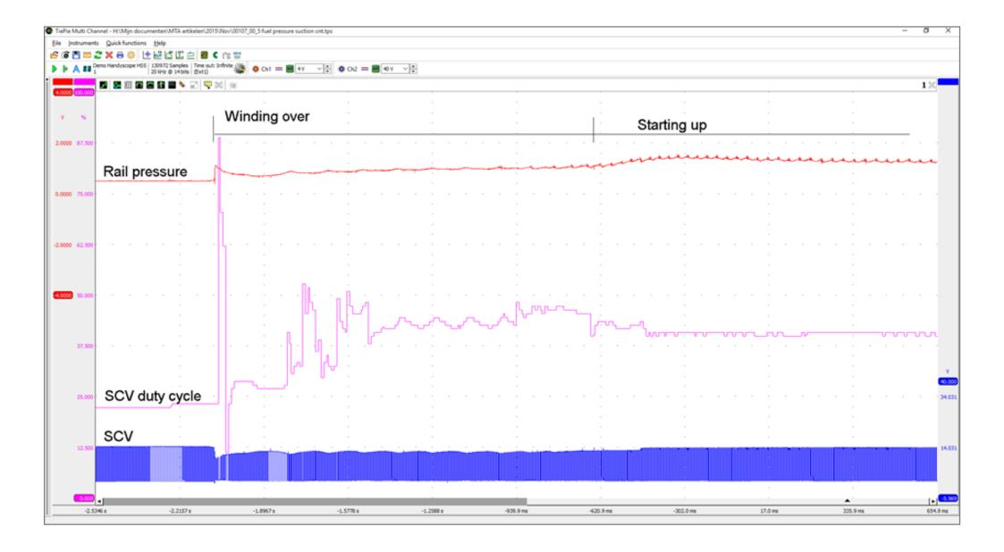
Picture 2: ATS recording of Rail pressure vs suction control valve (SCV).
