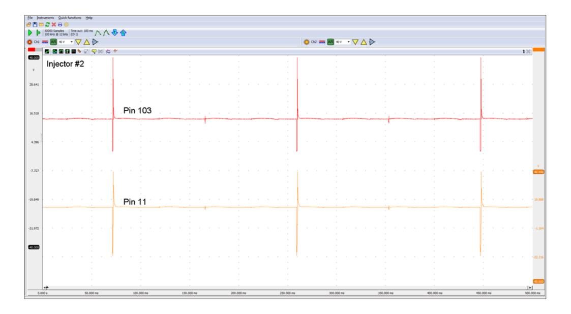
Picture 2 : ATS scope recording on injector 2
