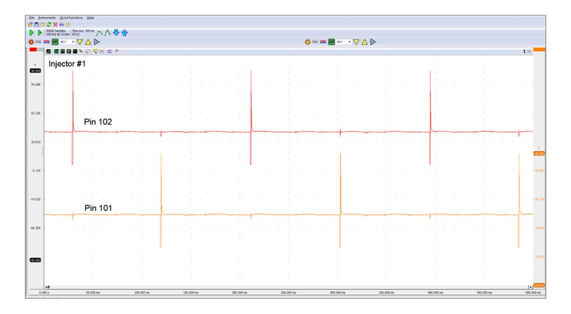
Picture 1: ATS scope recording on injector 1
