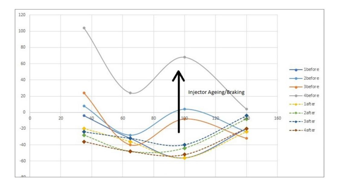
Figure 5: before and after replacement injector compensation results.
