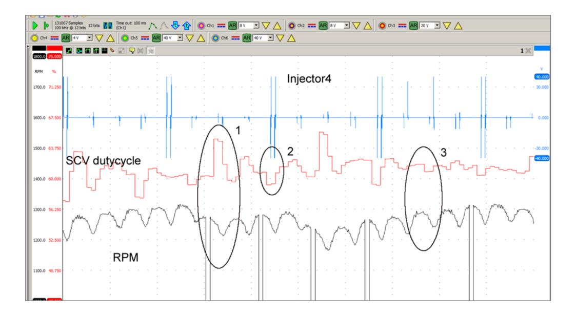
Figure 4: ATS 5004d scope recording of inj, SCV duty cycle and RPM.
