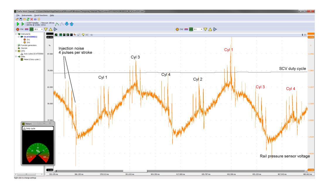
Picture 3 -ATS scope recording of rail pressure vs Duty cycle zoomed in. The pressure waves are in synch with the engine but out of phase with any one particular cylinder or injector
