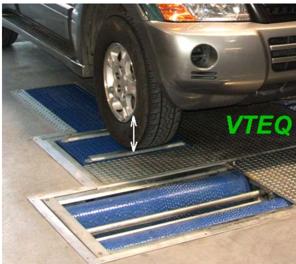
VTEQ test lane with car on the suspension tester
